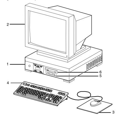
Figure 2-1. Components of the Sun Ultra 2 workstation
